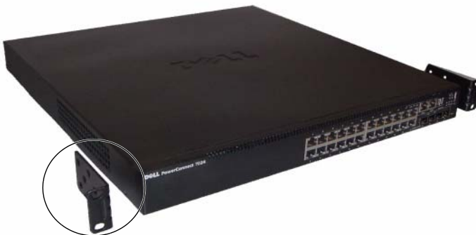
Figure 1-11. Fixation des supports
