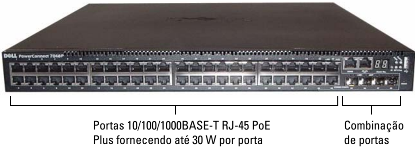
Figura 1-5. PowerConnect 7048P com 48 portas 10/100/1000BASE-T PoE Plus
